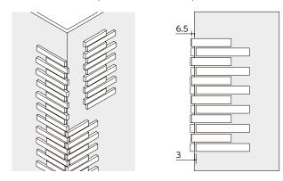
An external corner can be tiled with combinations of External Corner Starter Units and their vertically flipped Units (brick joint). Allow a joint width of 3 mm between the back faces of each unit and side faces of the combined units.
