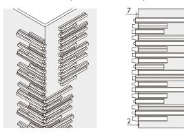
An external corner can be tiled with combinations of External Corner Starter Units and their vertically flipped Units. Allow a joint width of 2 mm between the back faces of each unit and side faces of the combined units.
