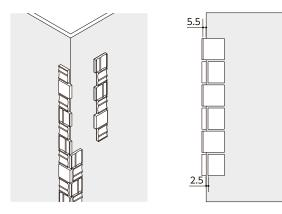
An external corner can be tiled with combinations of External Corner Starter Units and their vertically flipped Units. Allow a joint width of 2.5 mm between the back faces of each unit and side faces of the combined units.
