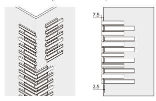
An external corner can be tiled with combinations of External Corner Starter Units and their vertically flipped Units (brick joint). Allow a joint width of 2.5 mm between the back faces of each unit and side faces of the combined units.
