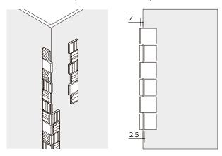
An external corner can be tiled with combinations of External Corner Starter Units and their vertically flipped Units. Allow a joint width of 2.5 mm between the back faces of each unit and side faces of the combined units.
