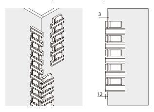
An external corner can be tiled with combinations of External Corner Starter Units and their vertically flipped Units (brick joint). Allow a joint width of 3 mm between the back faces of each unit and side faces of the combined units.
