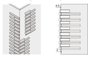
An external corner can be tiled with combinations of External Corner Starter Units and their vertically flipped Units (brick joint). Allow a joint width of 2 mm between the back faces of each unit and side faces of the combined units.
