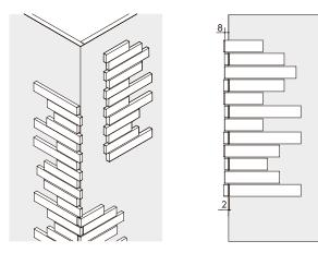
An external corner can be tiled with combinations of External Corner Starter Units and their vertically flipped Units. Allow a joint width of 2 mm between the back faces of each unit and side faces of the combined units.
