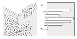
An external corner can be tiled with combinations of External Corner Starter Units and their vertically flipped Units. Allow a joint width of 2 mm between the back faces of each unit and side faces of the combined units.
