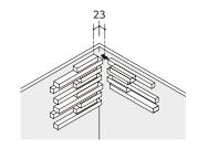
External Corner Starter Units can also be used to tile internal corners. Set recessed tile of both units 23 mm from the internal corner. Since the bedding is visible from between the gaps of the tiles, apply adhesive to the corner ends.
