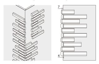
An external corner can be tiled with combinations of External Corner Starter Units and their vertically flipped Units. Allow a joint width of 4 mm between the back faces of each unit and side faces of the combined units.
