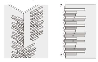
An external corner can be tiled with combinations of External Corner Starter Units and their vertically flipped Units. Allow a joint width of 2 mm between the back faces of each unit and side faces of the combined units.
